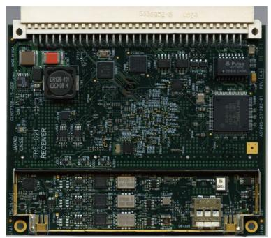
controllers. In addition, the board comes with large amount of flash for data storage. The CAN interface in TRE-G2T board is provided complete with all associated hardware and firmware, not just the CAN bus. The same is true with all the serial RS232/RS422 ports in our board. Simply stated, additional functions are not needed to incorporate any of our TRE-G2T OEM board in most applications.
