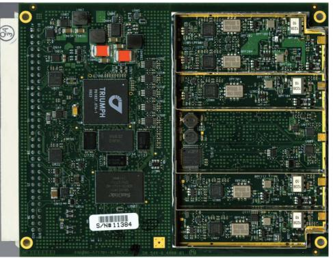
base. The other three receivers each track 14 each of GPS L1/L2, and Galileo E1 and along with the main one can provide attitude (orientation) solutions.
