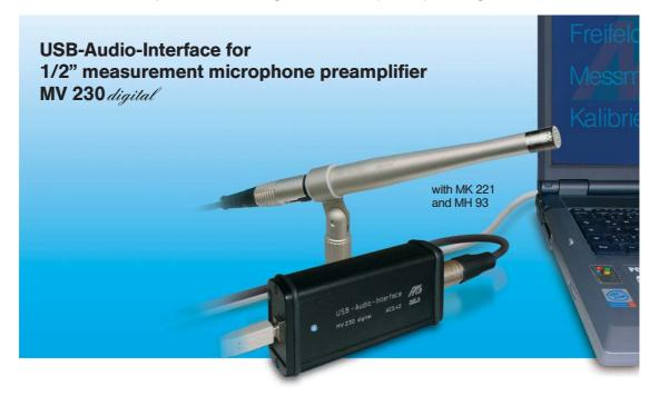
The system consists of the MK 221 measurement microphone capsule **MV 230** *digital*, measurement amplifier, 3-pin XLR-connecting cable, digital USB audio interface and a USB cable. Using an internal polarization voltage of 200 V, all measurement capsule can be used for either free or diffuse field operation within the audible, infrasonic or ultrasonic ranges (1 Hz to 40 kHz), encompassing the lowest to the highest levels.
