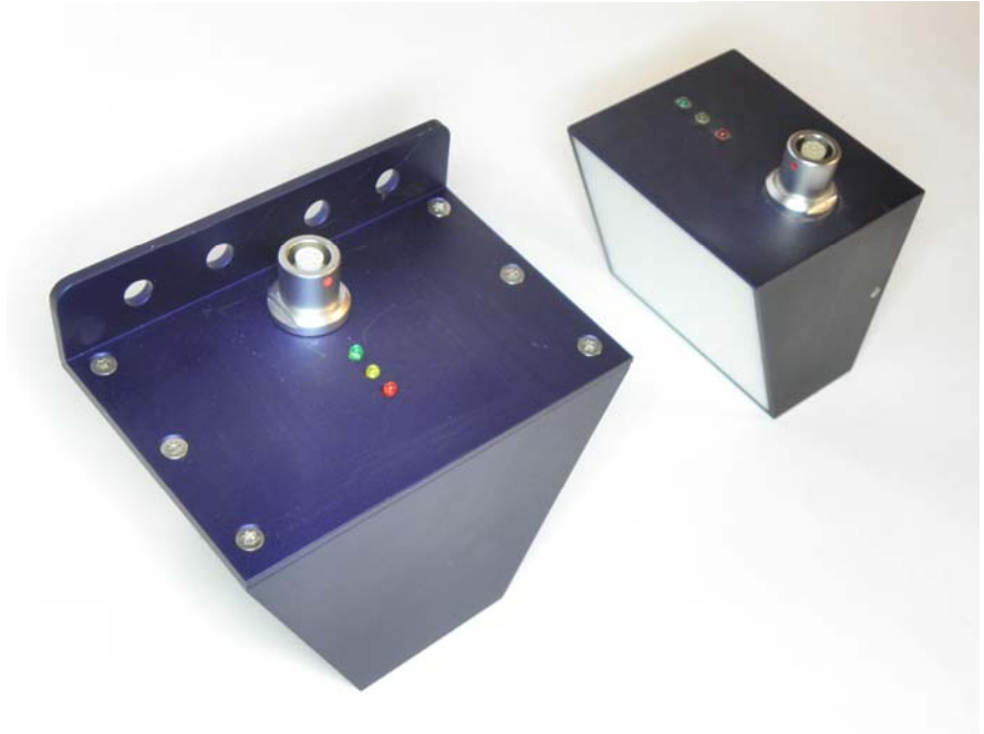
GSS25 (left) and GSS15 microwave Doppler sensors for speed over ground
