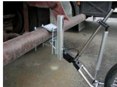
5 th - Wheel mounted at the rear protection bar
