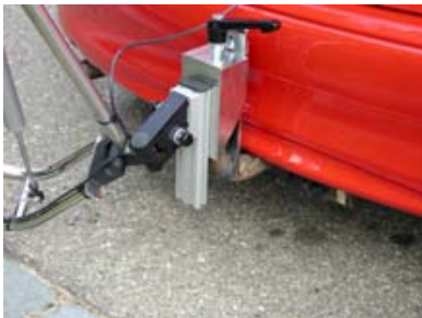
Attachment to the ball shaped trailer hitch
