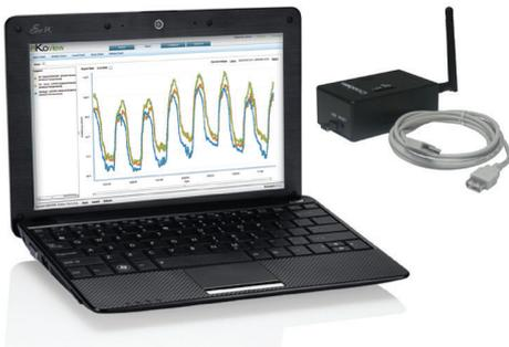
The eKo base station consists of three components- the eKo base radio, the eKo gateway and the eKoView web application
