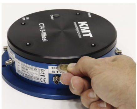
To lift the cover, use the slot!
