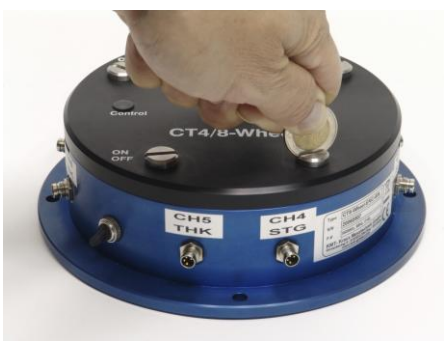
Untwist to open the housing, screws e.g. with coin!
