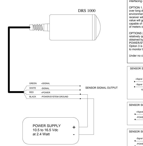
The signal output from the DRS1000 speed sensor is a 0 to 5 volt differential line driver that meets RS485 specifications. This type of output driver may be interfaced to the monitoring electronics in a number of ways. Three interfacing options are shown.
