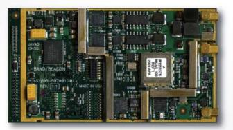
AW L-Band/Beacon OEM Receiver comprises two radio sections: L-Band receiver (1525 MHz to 1559 MHz) and Marine Radiobeacon receiver (283.5 to 325 kHz).
