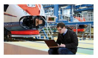
Multichannel measurements are common in railway applications, for example. imc allows decentralized, distributed and synchronous data acquisition involving thousands of channels – both inside and outside the rail vehicle. Due to the intelligent interaction with software solutions, the user obtains real-time results and can easily create reports.
