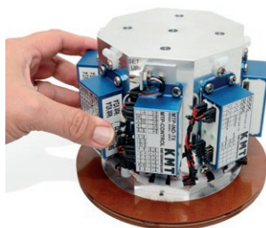
Telemetry for train wheel-set test bench
