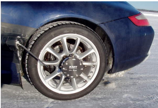
Force measurement on a car wheel with CTP-Rotate
