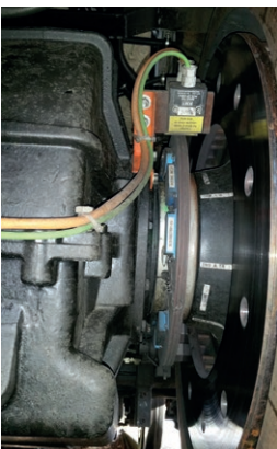
Force measurement on railway wheel set
