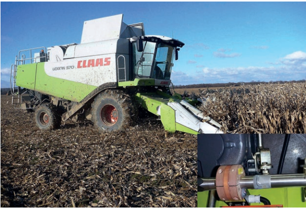
Torque measurement on combine harvester
