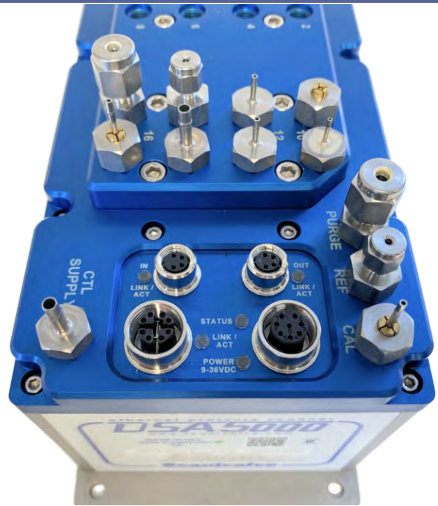
*SAE J1926-1 is equivalent to ISO 11926-1 for 5/16"x24 o-ring sealing straight thread fittings.
