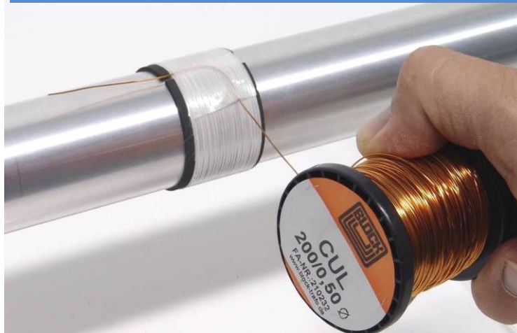
Coil, depends of shaft diameter 8-13 parallel windings of 0.5 CUL wire
