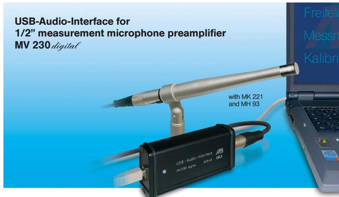
The system consists of the MK 221 measurement microphone capsule **MV 230 *digital***, measurement amplifier, 3-pin XLR-connecting cable, digital USB audio interface and a USB cable. Using an internal polarization voltage of 200 V, all measurement capsule can be used for either free or diffuse field operation within the audible, infrasonic or ultrasonic ranges (1 Hz to 40 kHz), encompassing the lowest to the highest levels.
