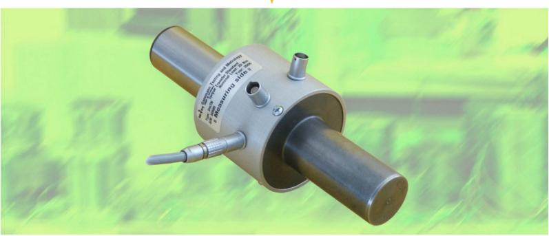
Transfer standards for comparison measurements of torque standard machines and for use as reference standards for the calibration of torque testing machines
