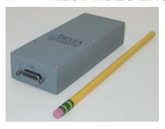
Delta's Model 6005R H.264 Video Encoder provides for the transmission of full-motion video for ISR applications. Primarily designed for small aircraft, the 6005R is a rugged, compact unit with all the features of Delta's JITC certified video encoder products. These include video compression, metadata processing and transport stream multiplexing.
