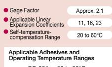
CC-33A: -50 to 80°C EP-34B: -50 to 80°C EP-18: -50 to 80°C
