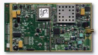
DSP based OEM Radio Transceiver with Built-in wireless link Monitoring and Management Tools:
