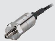
Highest accuracy in sub-miniature package Total error band from  $\pm$  0.1% to  $\pm$  0.5% fs according to temperature range Available from –55°C up to +150°C 0.5-4.5V signal with 8-30V DC power supply
