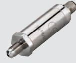
Pressure transducer with digital outputs Available with several protocols: CANbus, Modbus (...) High accuracy by linearization and polynomial correction over the compensated temperature range
