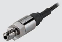
High temperature sub-miniature transducers Operating temperature -40°C to +175°C Amplified output: 0.5-4.5V DC Sub-miniature and ultra light sensor (all titanium) Very robust design
