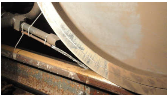
“Bad weather at the push of a button” thanks to the irrigation system directly before the front axle. © Photo: SBB
