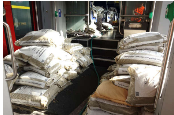
To substitute for the weight of passengers, the trainset was outfitted with sandbags. © Photo: SBB
