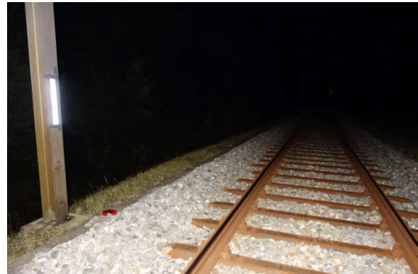
Using reflectors and beam sensors, the speed and distance signals can be double-checked during the test runs, and errors, such as a misaligned sensor, can be detected. © Photo: SBB
