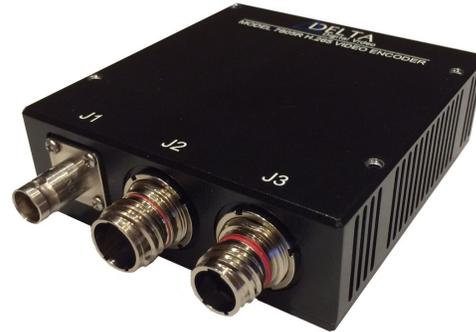
Delta's Model 7805R H.265 HD/SD Video Encoder provides for the transmission of full-motion video for ISR applications. Designed for operation in harsh environments, the 7805R is a rugged, compact unit with all the features of Delta's MISB/JITC certified video encoder products. These include, standards-compliant video compression, KLV metadata processing, and transport stream multiplexing.
