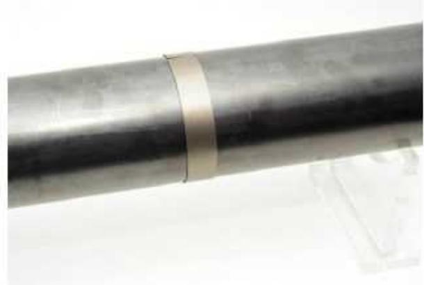
Attach for electromagnetic isolation "Ferrite Tape" 2 x one layer around the shaft.
