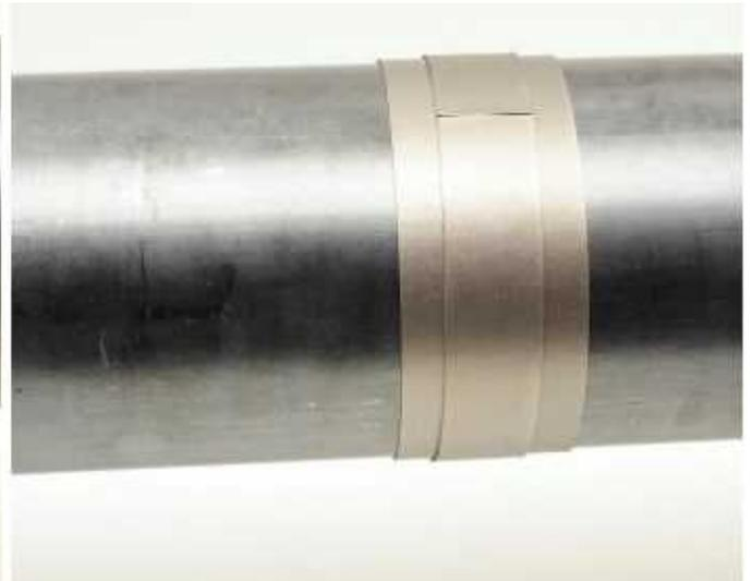
Attach for electromagnetic isolation "Ferrite Tape" 2x parallel and 1x in the middle over two layer around the shaft
