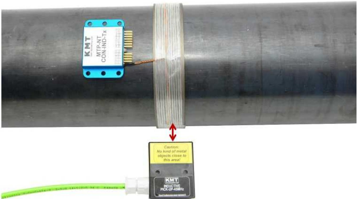
Inductive Pick-Up head mount in this position! Distance between head and Tx coil can be up to 50 mm, distance deepens of application.
