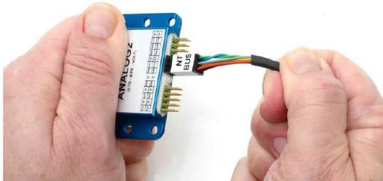
Caution: Locking-Clip must be completely connected!
