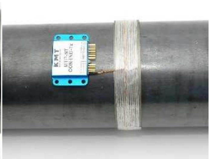
Extend the CUL wire flexible 0.14-0.25 mm (to decouple the inflexible 1 mm wire, at 0.63 not necessary) Twist also the flexible wire and solder it on the MTP-NT IND-Tx (isolate all solder points with shrink tubing)
