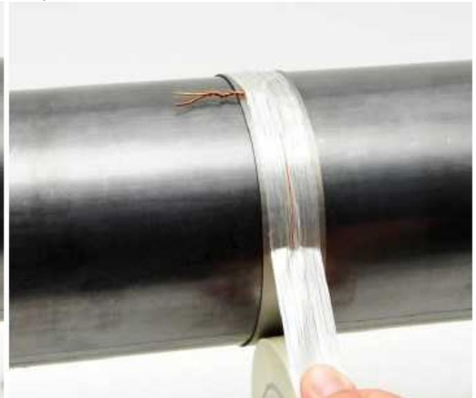
Make transmitting coil with 1x winding and twist the end of wire. Use CUL 0.63-1.00 mm wire
