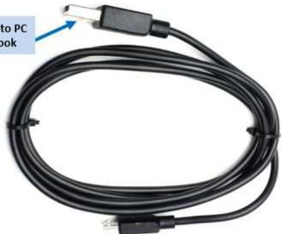
When connecting the USB port, a Windows COM port is created automatically. A driver doesn't have to be installed; we use the FTDI FT230X chip, which is always automatically recognized by Windows.
