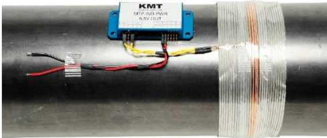
**Note:** "The inductive load of the MTP-NT IND-PWR and the capacitor in the Power Head must be in resonance to get the optimal transmission. The inductive load of the shaft depends of diameters, material and number of windings!
