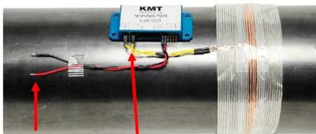
The pins "Coil" are the AC power input from the coil. On the pins "+6.5" and "GND" you get a stabilized output voltage of 6.5 V DC.
