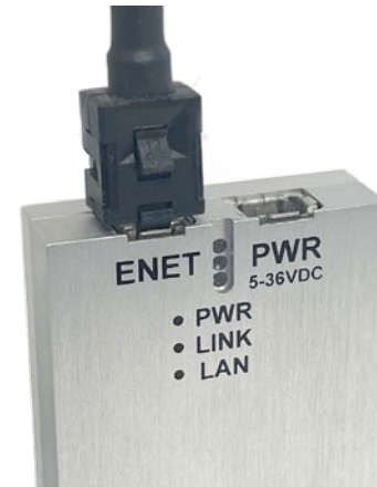
FIGURE 2-3: POWER & ETHERNET CONNECTIONS
