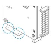
4) In the same manner, return the Alarm Module and attach to the end and fasten the center down with screws. (Recommended tightening torque: 4kgf/ cm). Tighten the upper screws first then the lower screws.
