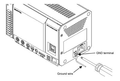
\* In order to prevent an electric shock and a fire, please ground the instrument using a GND terminal. For grounding, use a ground wire with a diameter of at least 0.75 mm<sup>2</sup>.
