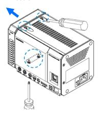
Slide the Amplifier Module parallel to the GL7000 and connect.
