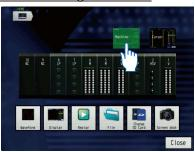
Since this is a capacitive touch-screen, mechanical device such as a pen or pencil will not work. Remove gloves etc. and operate it with your fingers.
