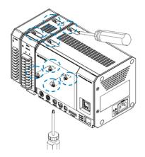
\* When installing multiple modules, install one at a time. Make sure to fasten with screws before installing the next module.
