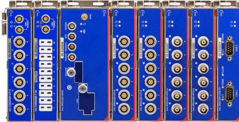
Based on an imc ARGUSfit base unit, imc ARGUSfit measurement amplifier and interface modules can be combined to form complete systems by means of a robust click mechanism, which can even integrate imc CANASfit modules. The click connectors provide the electrical connection to the power supply and system bus.
